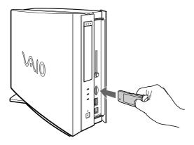
Hold the Memory Stick<sup>TM</sup> with the arrow pointing in the correct direction when you insert it into the slot. To avoid damaging the computer or the Memory Stick<sup>TM</sup>, do not force the Memory Stick<sup>TM</sup> into the slot if it does not insert smoothly.
